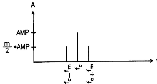
FIGURE 4.14 Spectrum of the AM signal produced by the instrument of figure 4.13.
